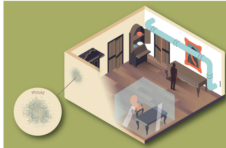
Figure 13: Changing the moisture content or the temperature of the indoor air can increase the risk on the outside of the building. Ducts will negatively affect the experience of a historic interior, while placing objects inside a display case will affect the way visitors view the objects.
